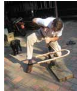
Step 4: Drill 3/8" holes (30 holes/shoe; brace & bit)
