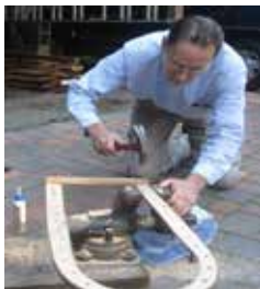
Step 5: Attach tail brace (cut, drill, glue, dowel;)
